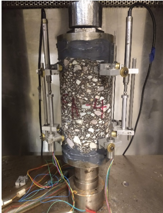
Cyclic Fatigue Test
