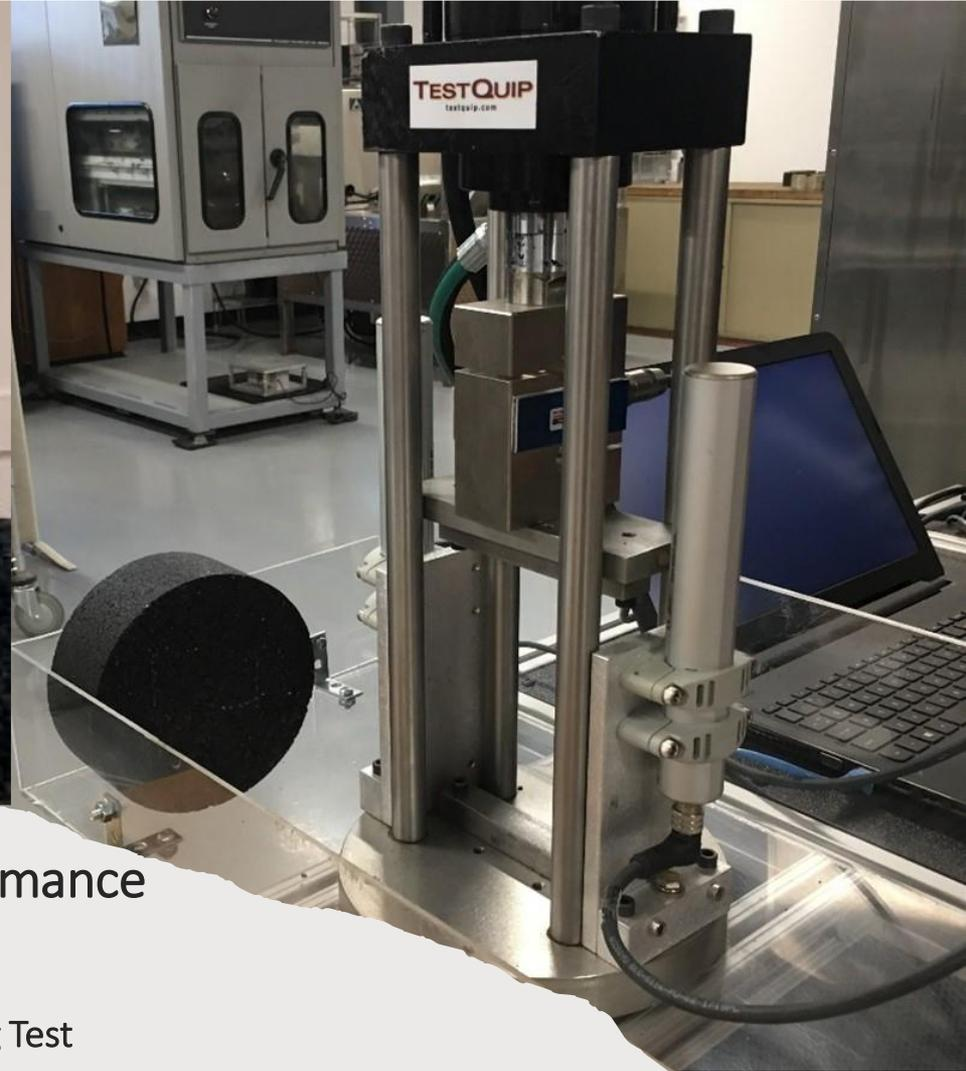
Balanced Mix Design – Tests mix for performance related to rutting and cracking resistance.
