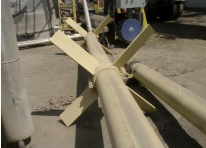
Tanks require mixers - Low shear tank mixer
