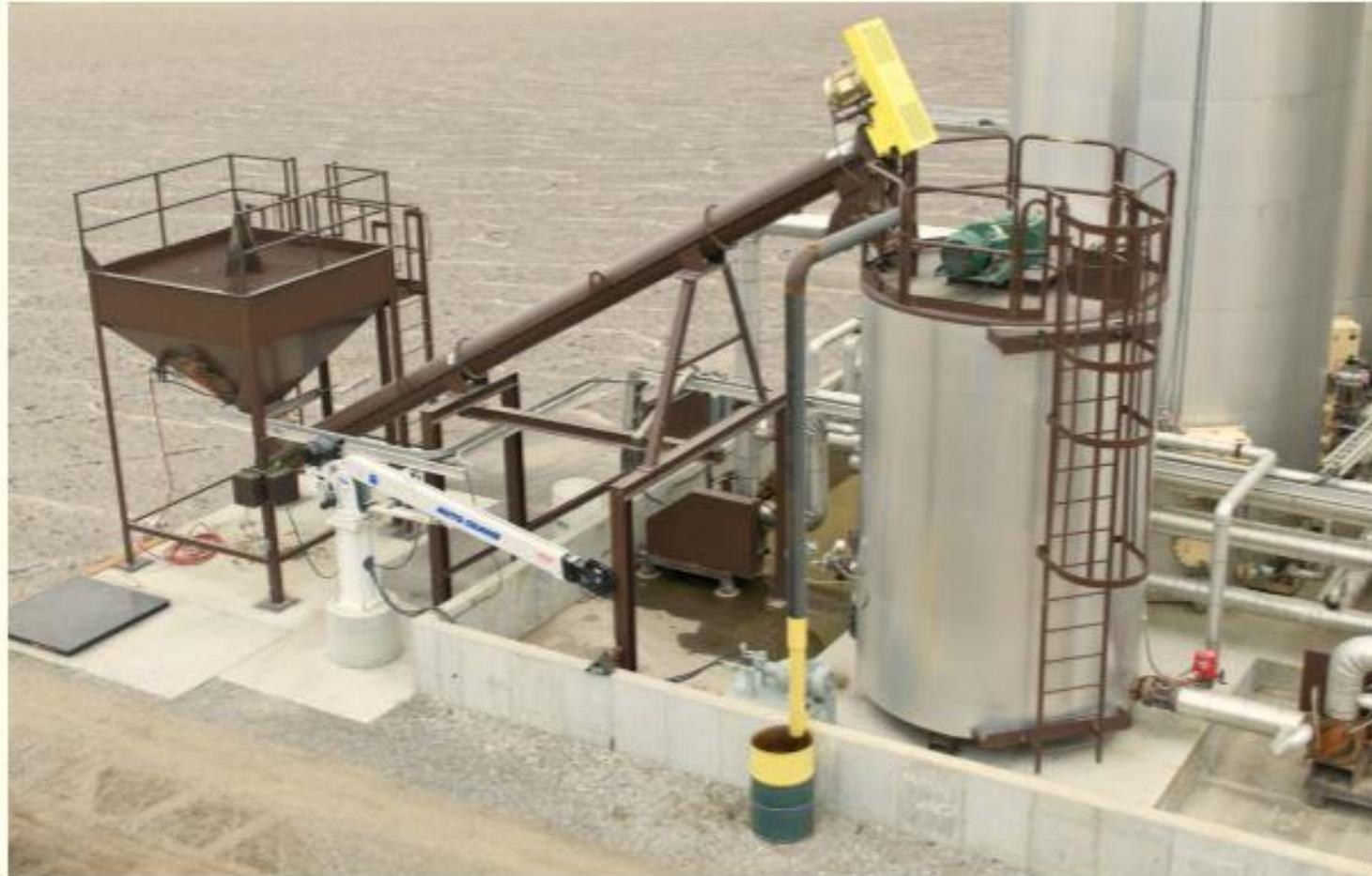
Rubber feed hopper, batch method
