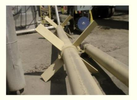
Tanks require mixers - Low shear tank mixer
