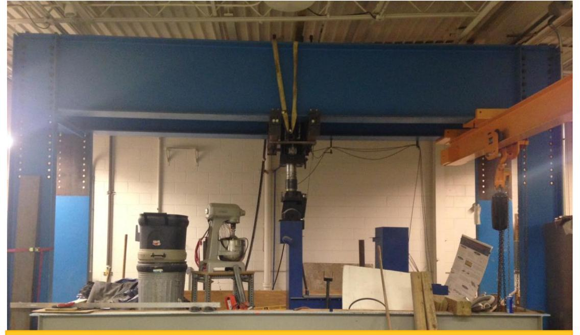
Large-scale testing facility for slab experiments
