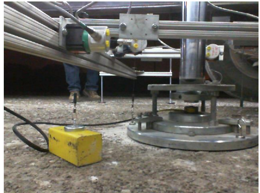
Subbase/Subgrade Composite M_r = 25,162 psi
