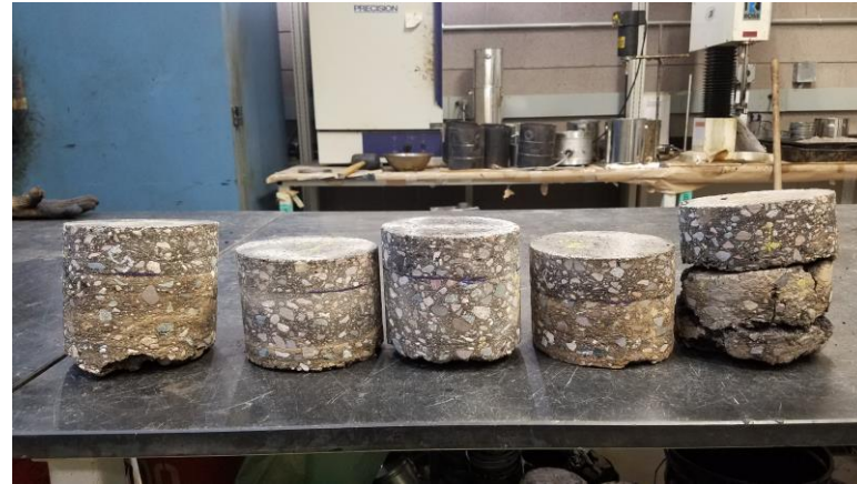
Cores taken from 15% RAP Section
