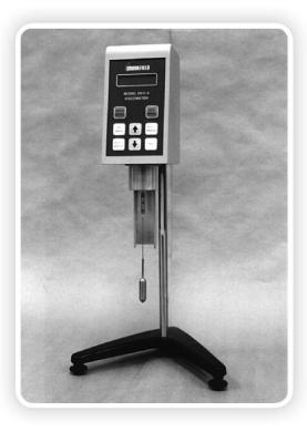
Superpave adopted AI procedure using rotational viscometer
