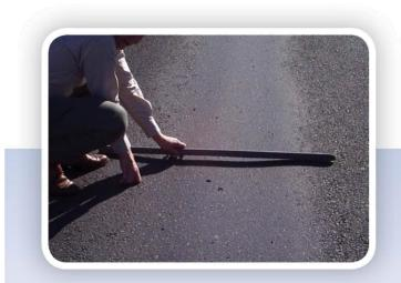
PG 67-22 Unmodified Asphalt 15mm rutting
