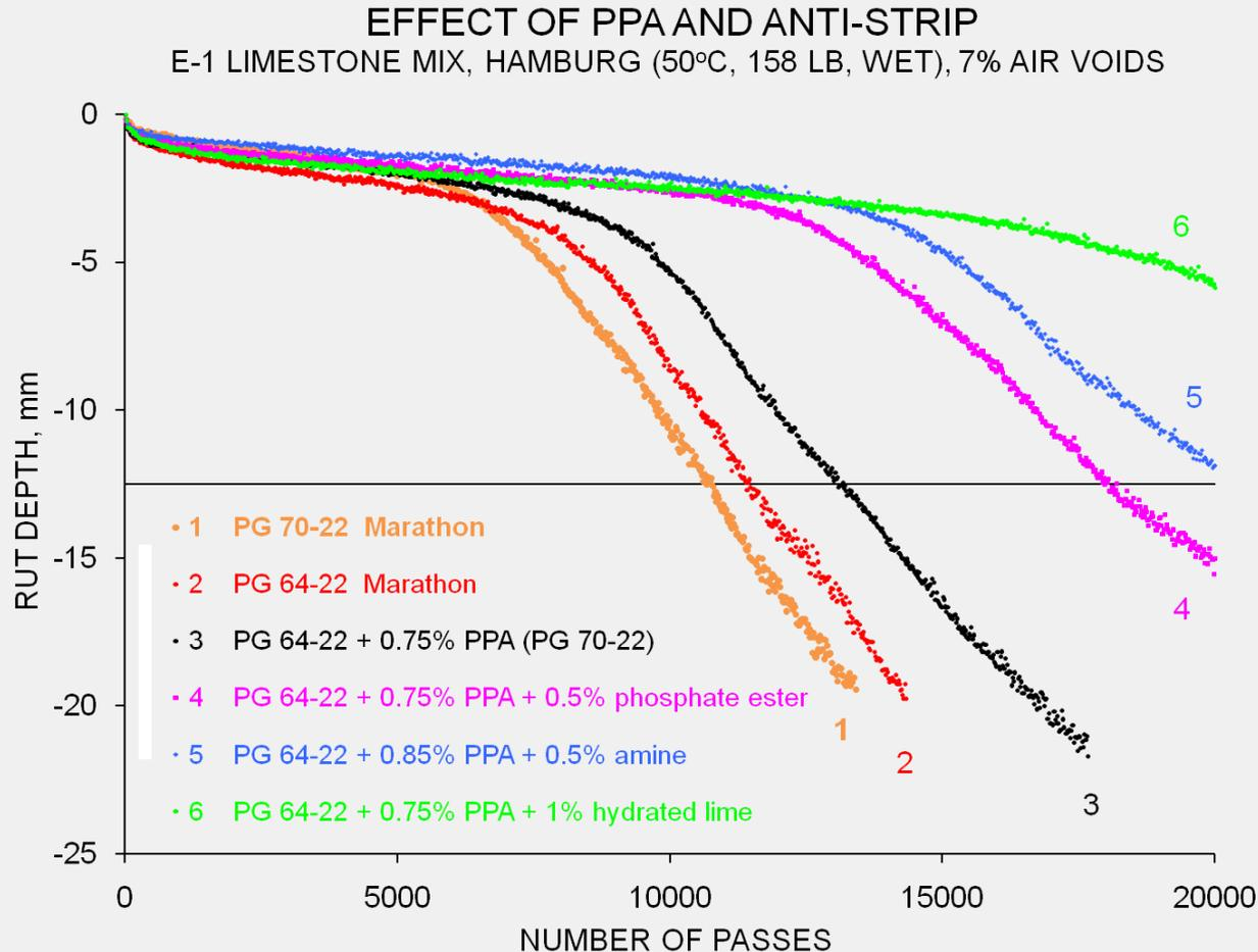
PPA performs well with proper anti-strip. Need to test all mix components.
