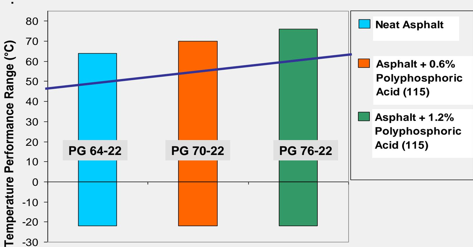
Polyphosphoric Acid increases the high-temperature grading with no loss of the low-temperature properties
