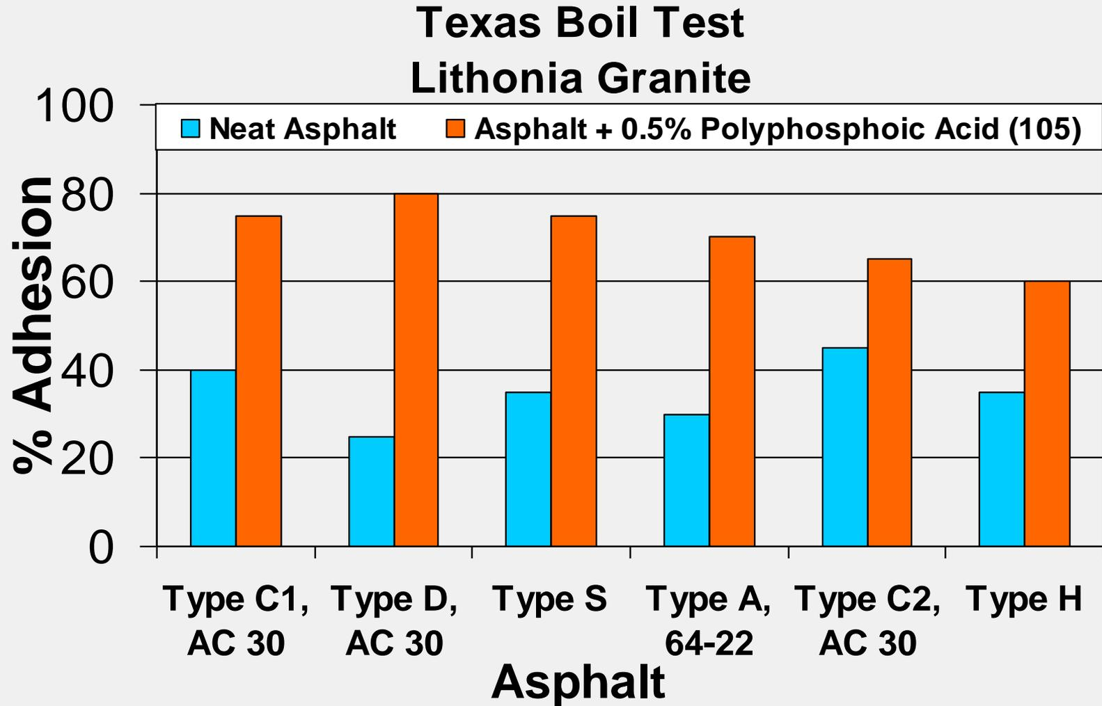
*Use of Polyphosphoric Acid results in improved adhesion vs neat asphalt*
