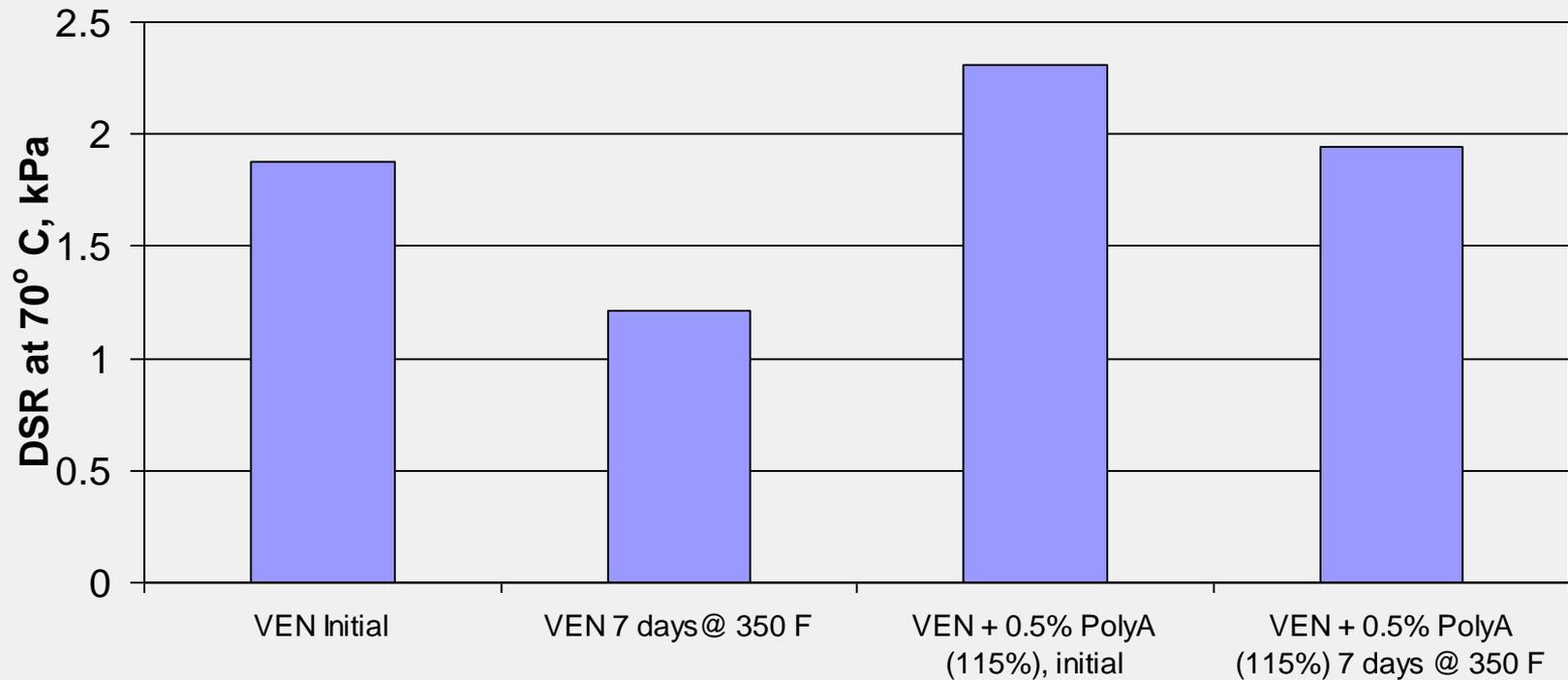
Under prolonged high-temperature storage, Polyphosphoric Acid results in an asphalt that maintains its PG rating.
