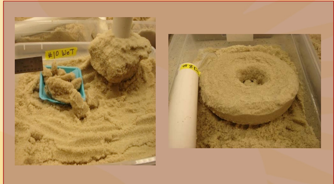
275-mm diameter, 19 liter bucket test w/ 50-mm diameter perforated pipe
