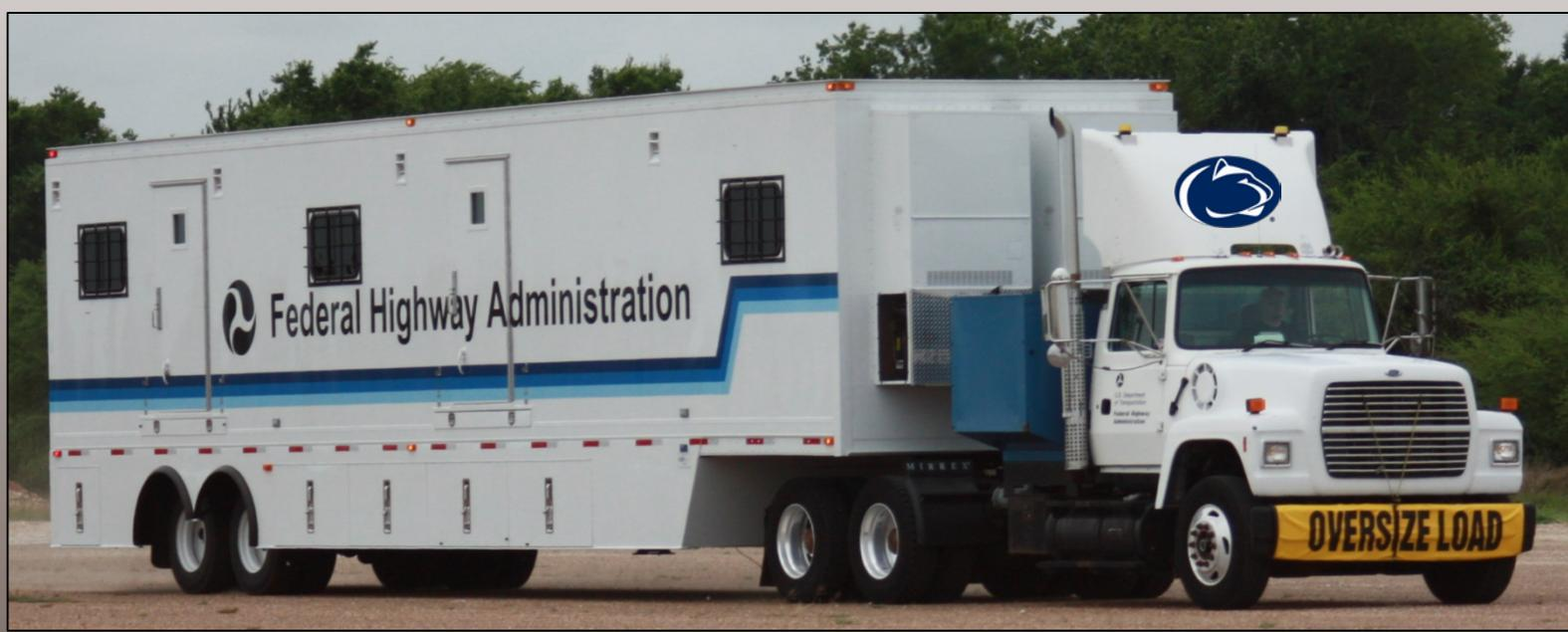
FHWA's Mobile Asphalt Testing Trailer
