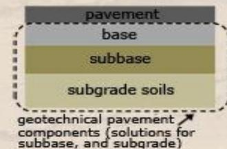
▶ Geotechnical Pavement Components (Base, Subbase, and Subgrade)
