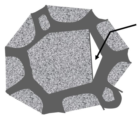
Separation of asphalt from aggregate
