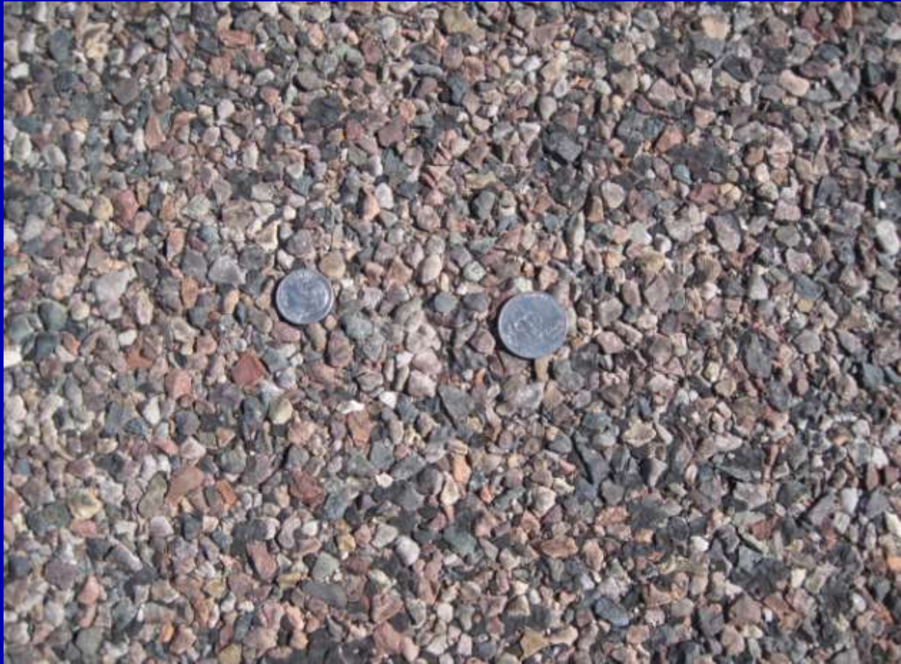
LV Chip Seal 1/4" Aggregate
