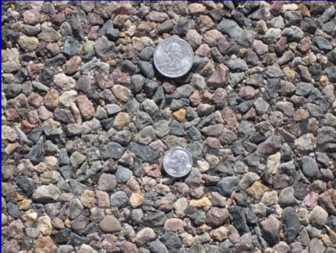
HV Chip Seal 3/8" Aggregate
