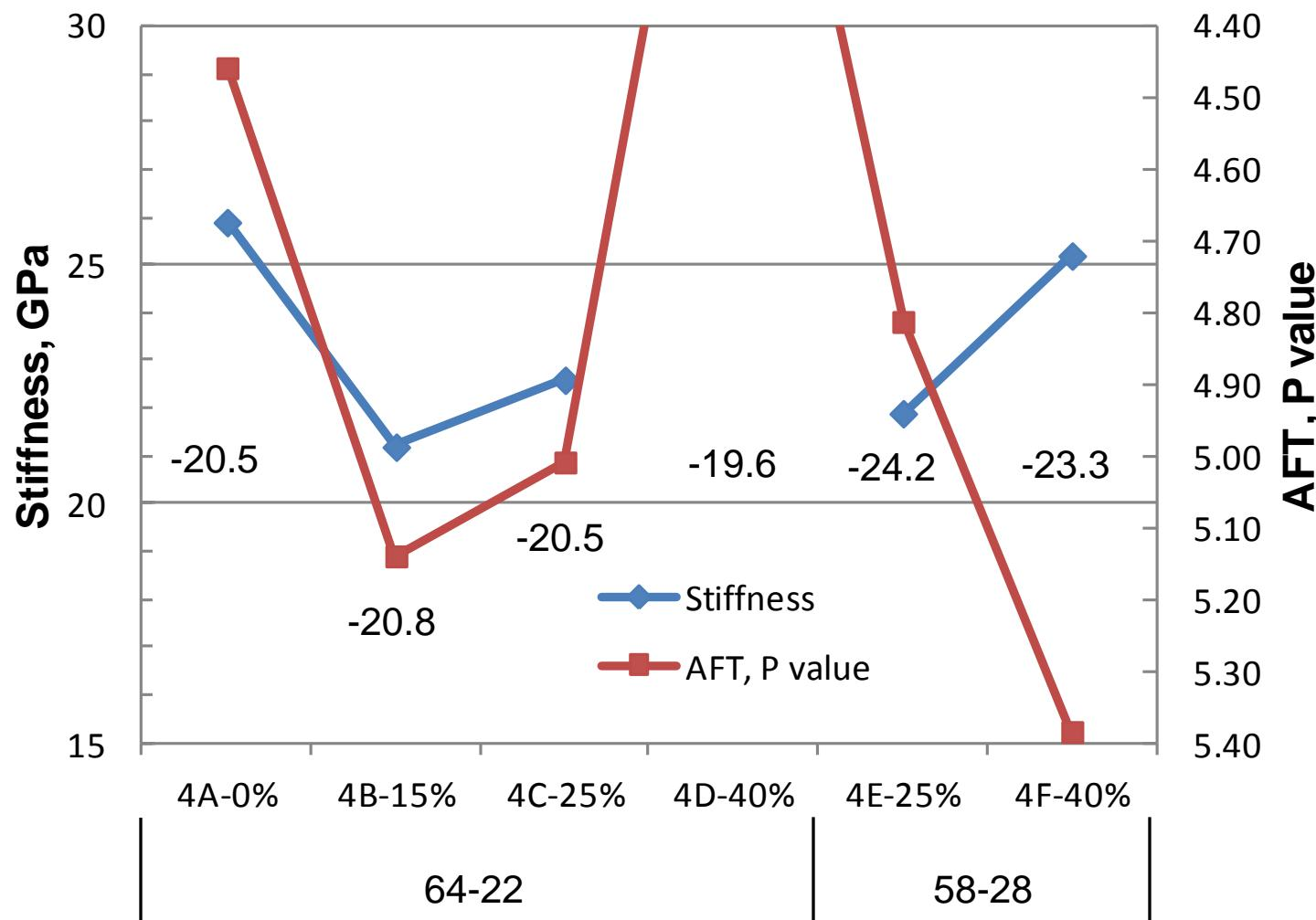
Stiffness data from: *Investigation of Low and High Temperature Properties of Plant-Produced RAP Mixtures Phase II*, McDaniel and Huber
