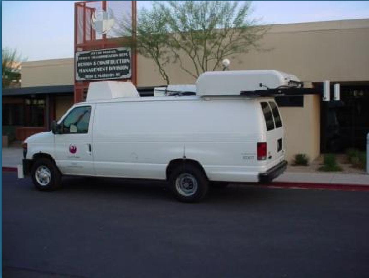
Pavement Management Van: Automatic Road ANalyzer (ARAN) van
