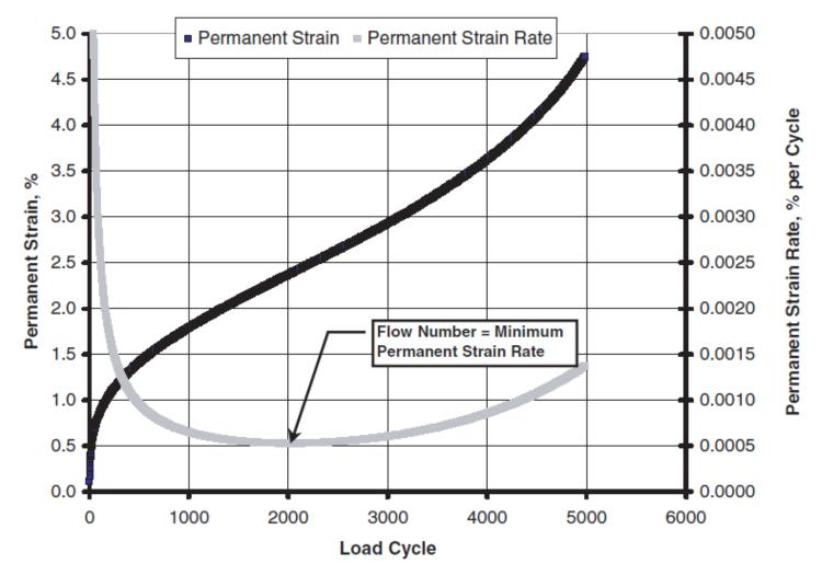
Figure 6-2. Typical data from the flow number test.
