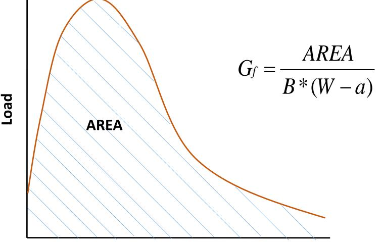
**Crack Mouth Opening Displacement (CMOD)**
