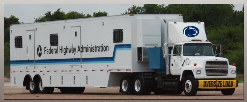
FHWA's Mobile Asphalt Testing Trailer Office of Asset Management, Pavement, and Construction
