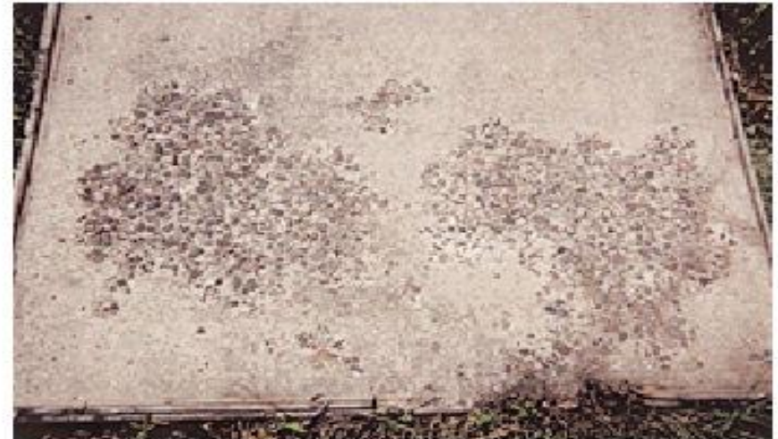
Fig. 8-3. Effect of weathering on boxes and slabs on ground at the Long-Time Study outdoor test plot, Project 10, PCA, Skokie, Illinois. Specimens at top are air-entrained, specimens at bottom exhibiting severe crumbling and scaling are non-air-entrained. All concretes were made with 335 kg of Type 10 (Type I) portland cement per cubic metre. Periodically, calcium chloride deicer was applied to the slabs. Specimens were 40 years old when photographed (see Klieger 1963 for concrete mixture information). (69977, 69853, 69978, 69854)
