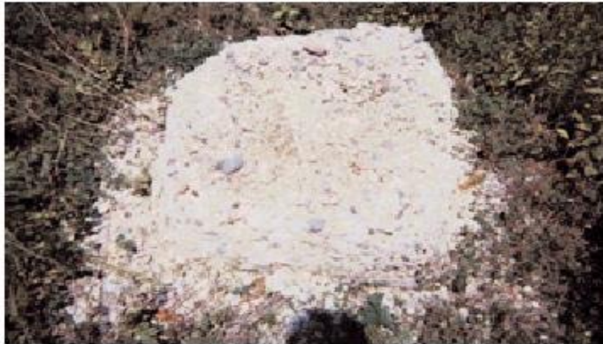
Fig. 8-3. Effect of weathering on boxes and slabs on ground at the Long-Time Study outdoor test plot, Project 10, PCA, Skokie, Illinois. Specimens at top are air-entrained, specimens at bottom exhibiting severe crumbling and scaling are non-air-entrained. All concretes were made with 335 kg of Type 10 (Type I) portland cement per cubic metre. Periodically, calcium chloride deicer was applied to the slabs. Specimens were 40 years old when photographed (see Klieger 1963 for concrete mixture information). (69977, 69853, 69978, 69854)
