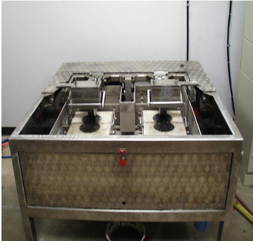
Hamburg Wheel Tracker capable of running two sets of specimens simultaneously
