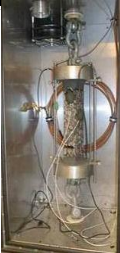
Specimen with acoustic emission sensors
