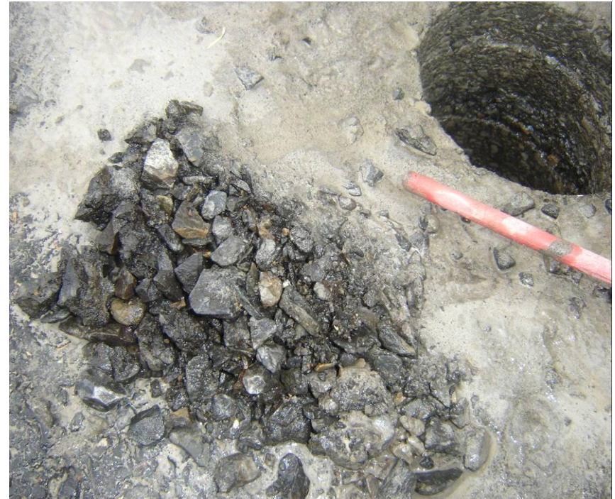
Severe stripping – the asphalt binder is gone
