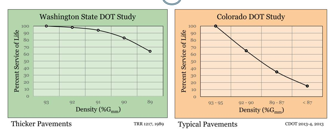
Reduced in-place density at the time of construction results in significant loss of service life!
