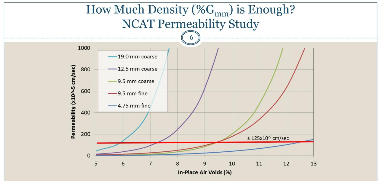
Finer NMAS mixes generally less permeable at equivalent air void levels!
