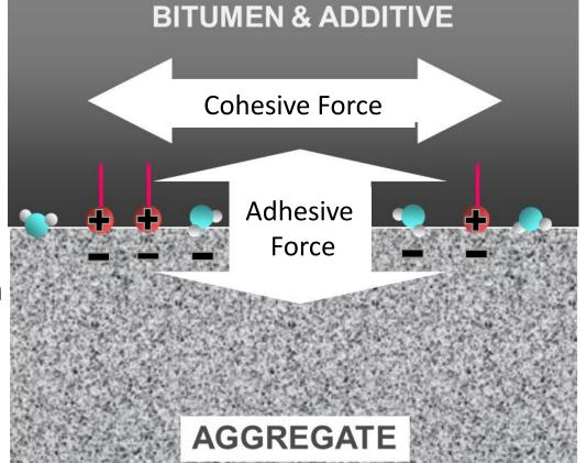
In colder temperatures, cohesive forces in the bitumen may cause the film to contract
